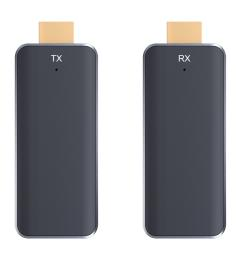
S101 includes one wireless sender and one wireless receiver. Plug the receiver with the TV, and connect the wireless video transmitter with the video source. The wireless video sender and receiver will pair automatically and start the transmission.
